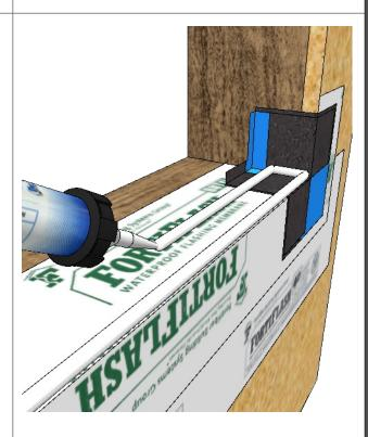
The **Ready Sill**® End Dam should be pressed into the wet **Moistop Sealant**® and J-Rolled into place. Place the **Ready Sill**® End Dam in the correct location based upon the window size you are using. Place the inside lip of the end dam so that it will be 1/8" back from the inside edge of the window.
